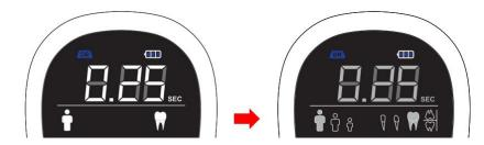
(2) To return to normal operation, press any key or the X-ray exposure button.
