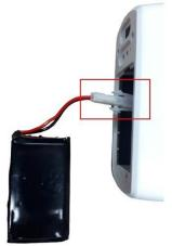
③ Install the new battery in the reverse order of removal.
