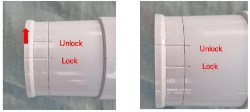
(2) Remove the collimator and backscatter shield ring as the below picture.
