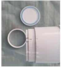
(3) Fastening backscatter shield and collimator as below picture. Lock the collimator by turning as the above (1) picture.
