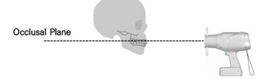
③ Place the cone of the portable dental x-ray system head in the area want to take an image. When holding the device, it is recommended to grip the handle by one hand and place the other on the underside of the Exposure Button and the cone as shown in the following figure.
