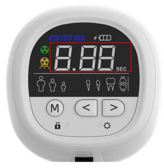
The X-ray exposure time can be set in the range of 0.02 to 0.5 sec and adjustment by 0.01 sec step.
